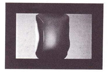
The  $>45^{\circ}$  edge angle of the oil drop remained absolutely unchanged during the test period of 6 months.
